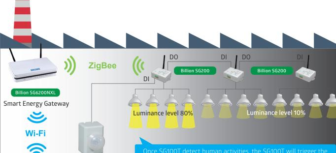
Once SG100T detect human activities, the SG100T will trigger the SG200 (Billion Lighting Control Box), which will adjust the lighting to reach the user's pre-configured luminance level. When in the situation SG100T detect no human activities, the SG200 will automatically dim the interiors lights to the lowest luminance level to minimize power consumption.
